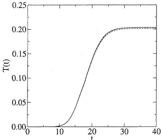
Fig. 4. Transmitted norms for a wave packet with  $K = 1.06$  incident on the three potentials. The curves correspond to the results obtained for the reference (solid line), “ears up” (dashed line), and “ears down” (dotted line) potentials.
