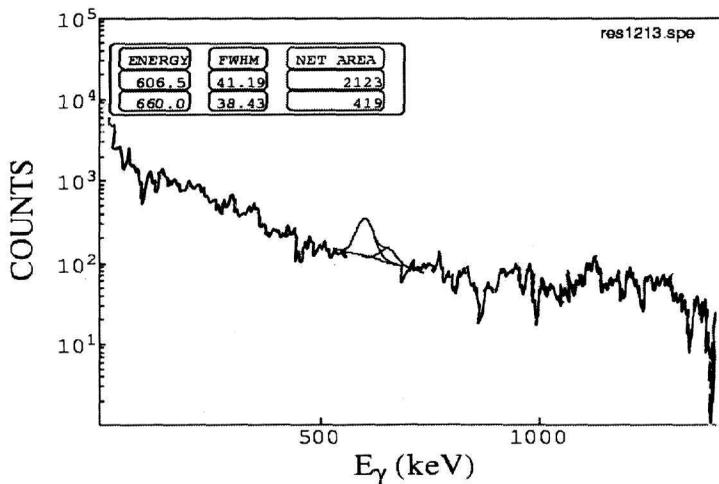
Fig. 4. The deconvolution result for separating the 609 keV (<sup>214</sup>Bi) contribution from 662 keV <sup>137</sup>Cs) in the gamma-ray spectrum on the 13<sup>th</sup> August 2001.
