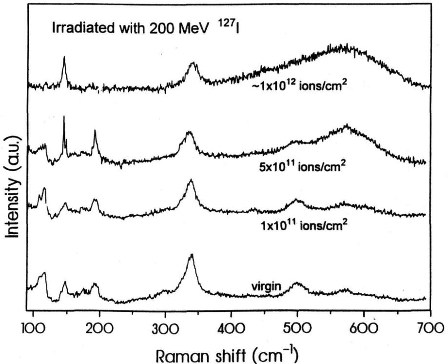
Fig. 3. Raman spectra of  $\text{YBa}_2\text{Cu}_3\text{O}_7$  films on MgO as deposited (virgin) and irradiated at three different doses with  $200\text{ MeV }^{127}\text{I}$ . The peak at  $190\text{ cm}^{-1}$  corresponding to the MgO substrate is not present in the upper spectrum (irradiation dose  $\sim 1 \times 10^{12}\text{ ions/cm}^2$ ) since the sample was thick enough so that the substrate could not be seen by the laser beam.
