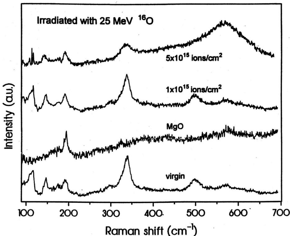
Fig. 2. Raman spectra of  $\text{YBa}_2\text{Cu}_3\text{O}_7$  films on  $\text{MgO}$  as deposited (virgin) and irradiated at two different doses with 25 MeV  $^{16}\text{O}$ . The Raman spectrum of the  $\text{MgO}$  substrate is also shown for comparison.
