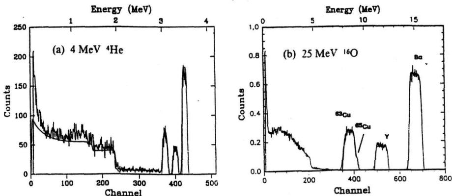
Fig. 1 . RBS spectra of  $\text{YBa}_2\text{Cu}_3\text{O}_7$  films on MgO, taken with 4 MeV  $^4\text{He}$  (a) and 25 MeV  $^{16}\text{O}$  (b). The solid lines represent simulation by RUMP code.
