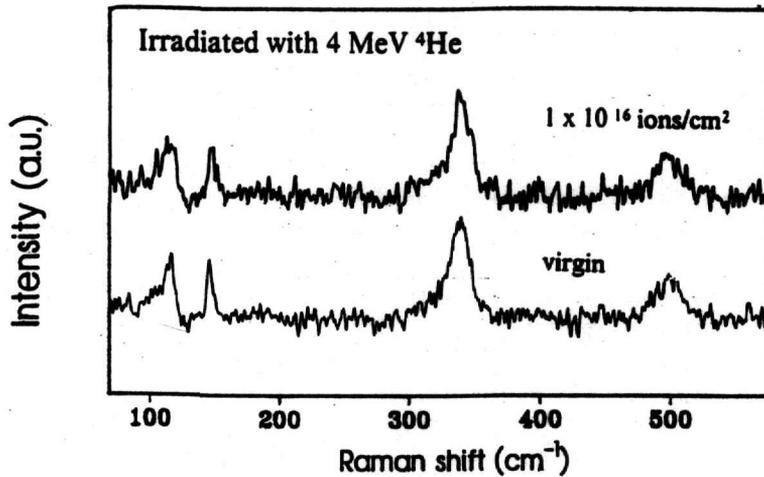
Fig. 4. Raman spectrum of YBa<sub>2</sub>Cu<sub>3</sub>O<sub>7</sub> films on MgO as deposited (virgin) and irradiated with 4 MeV <sup>4</sup>He.
