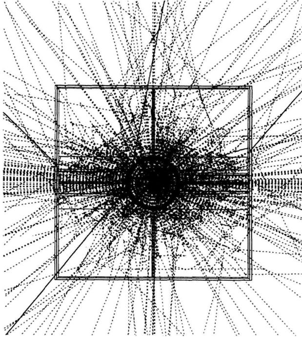
Fig.5 Simulation of 500 photons of 835 keV
