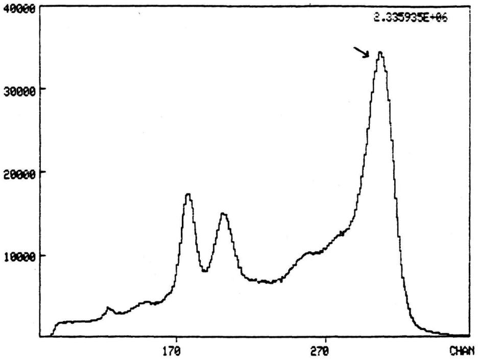
Fig. 3 Sum spectrum of a  $^{22}\text{Na}$  radioactive source
