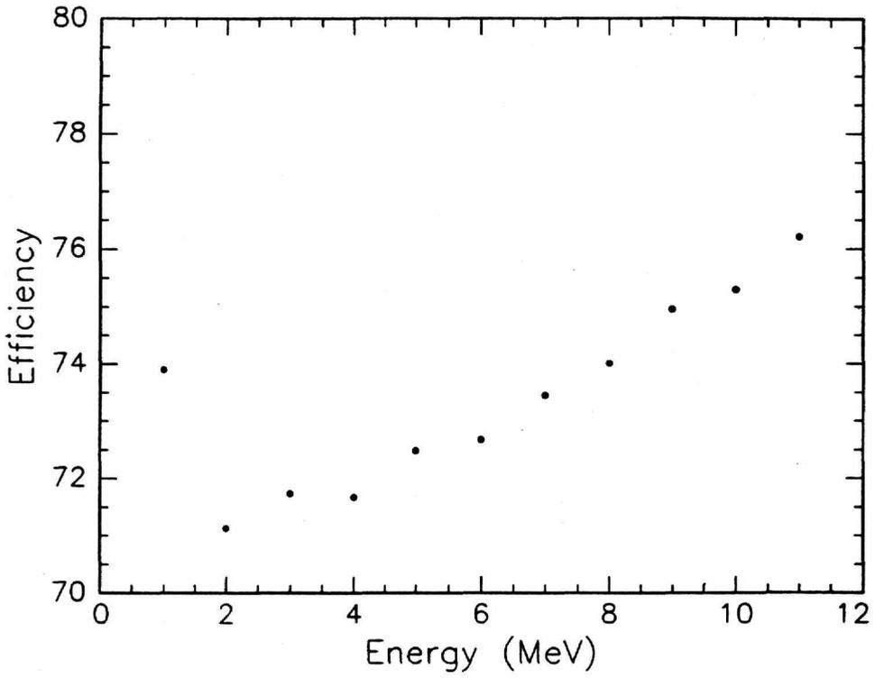
Fig.6 Efficiency of 'PTOLEMEOS' vs energy for monoenergetic photons
