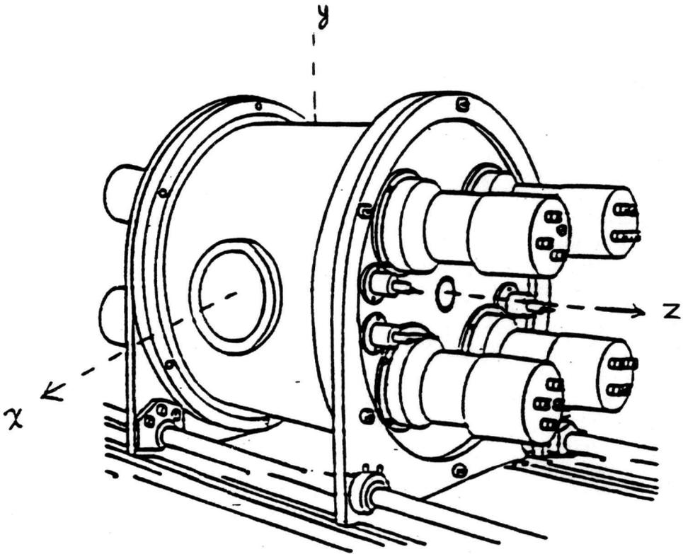
Fig.1  $4\pi$  NaI  $\gamma$ -ray detection system PTOLEMEOS
