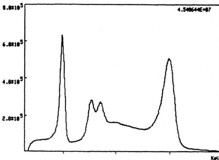
Fig. 2b Spectrum of  $^{137}\text{Cs}$  and  $^{60}\text{Co}$  sources taken with all the detectors active. Summing peak is highly increased.
