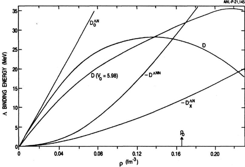
Fig. 6: The  $\Lambda$  binding  $D(\rho)$  and its components vs.  $\rho$  for an interaction with  $V_0 = 6.16 \text{ MeV}$ ,  $W = 0.01 \text{ MeV}$ ,  $C_p = 2 \text{ MeV}$ ,  $\epsilon = 0.34$  for which the s.p. energies are shown in Fig. 4. Also shown is  $D(\rho)$  for only  $V_{\Lambda N}$  ( $V_0 = 5.18 \text{ MeV}$ ) with  $\epsilon = 0.88$ .
