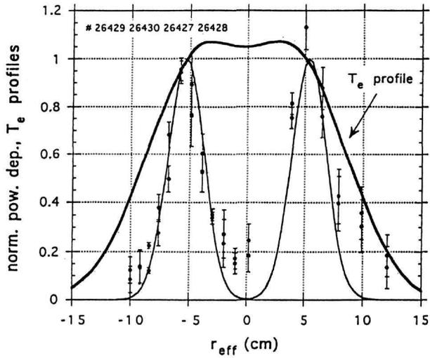
**Figure 4a:** The normalized electron temperature profile in comparison with the power deposition profile from a modulation frequency scan for off-axis power deposition. Measured data points for 2 and 4 kHz are included which are taken as the basis for the extrapolation.
