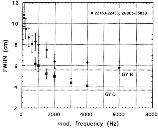
**Figure 2a:** The full width at half maximum (FWHM) of the Gauss fitted temperature modulation profiles as a function of modulation frequency for two different ECRH beamlines. The limiting values obtained by Lagrange extrapolation are given by the dotted lines labeled Gy B and GyD.
