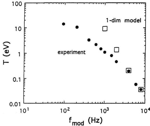
**Figure 6:** Modulation amplitude of the 67 GHz channel as function of modulation frequency in comparison with 1-D Fokker-Planck calculations. The deviation at low frequencies is due to diffusive transport which is being neglected in the model.
