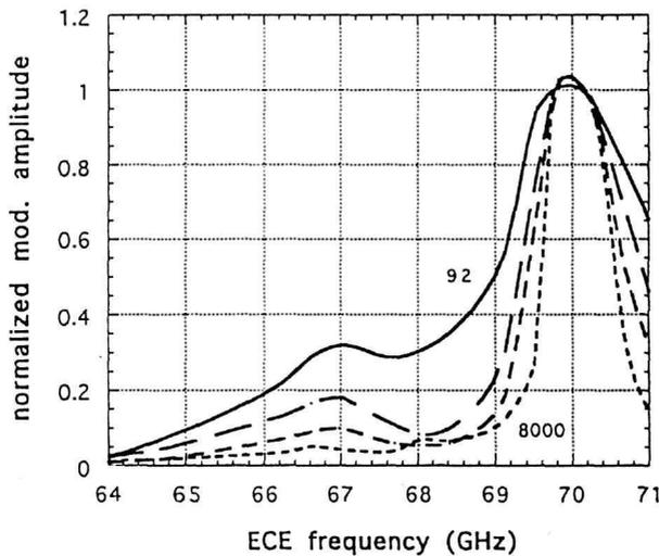
**Figure 5:** The normalized modulation amplitude as function of ECE frequency given for a sequence of modulation frequencies between 92 and 8000 Hz. The second maximum at the low frequency end of the spectrum corresponds to down-shifted non-thermal emission. It decays stronger with increasing modulation frequency than the thermal emission.
