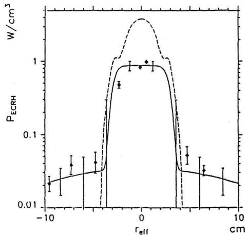
**Figure 3:** ECRH power deposition profile from transient power balance analysis (solid line) and least squares Lagrange extrapolation (dots) from a modulation frequency scan with special attention to the broad background deposition. For comparison the single path ray-tracing result is included (dashed line).
