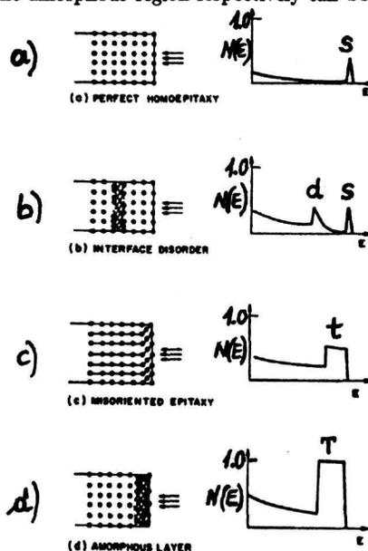
FIG. 5: Channeling spectra of epitaxial systems (from ref. [1]).
