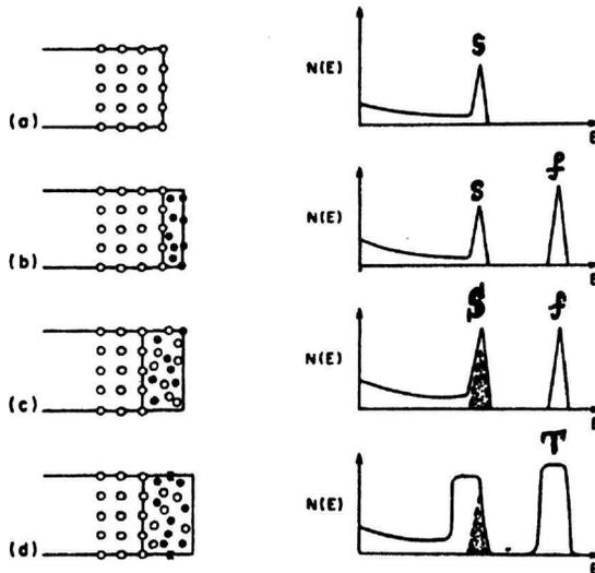
FIG. 4: Channeling spectra for amorphous film on single-crystal substrates.  $\circ$ :=atoms of crystal with mass  $M_2$ .  $\bullet$ :=atoms of the deposited layer of mass  $M_3$ . ( $M_3 > M_2$ ). (From ref. [1]).
