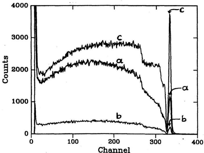
FIG. 15: RBS-spectra of a BaBiCuO surface layer bombarded with protons
