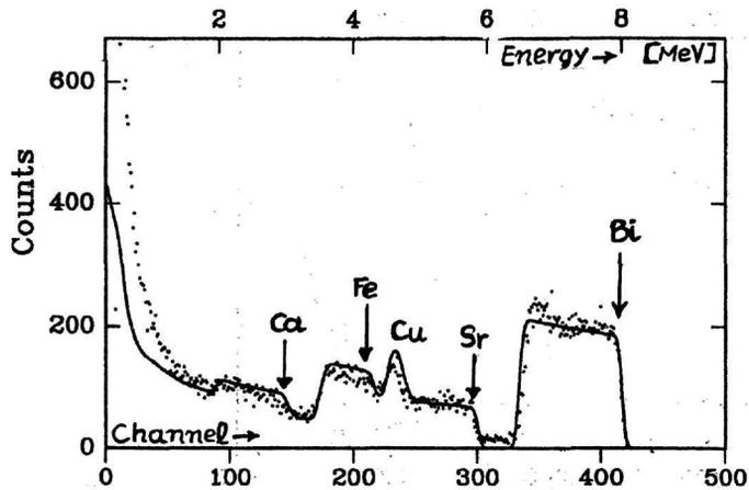
FIG. 20: Experimental ("dotted") and simulated ("solid") RBS-spectrum of a thick MgO substrate with a rather complex layer on its surface (see text).
