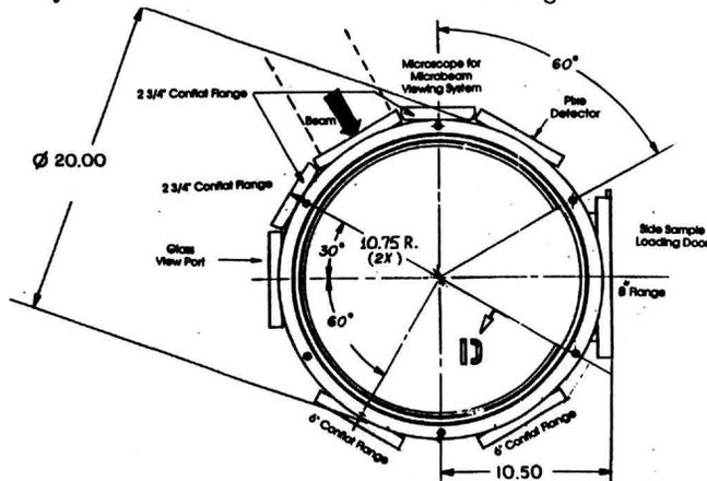
FIG. 8: Horizontal cut of the vacuum chamber.
