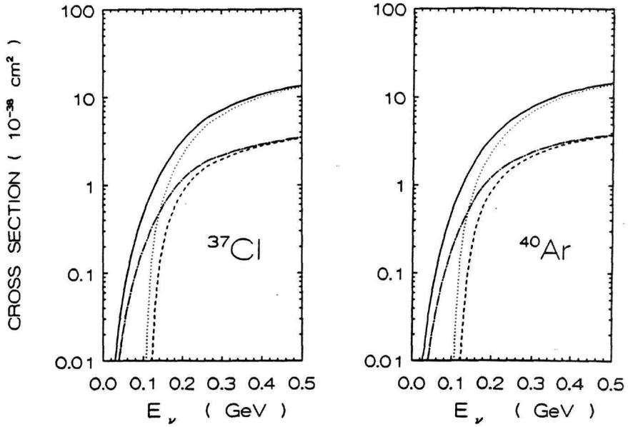
**Fig. 1:** Total cross sections for neutrino-nucleus reactions for  $^{37}\text{Cl}$  target (left) and  $^{40}\text{Ar}$  target (right). Graphs are:  $^{37}\text{Cl}(\nu_e, e^-)^{37}\text{Ar}$  (solid line),  $^{37}\text{Cl}(\nu_\mu, \mu^-)^{37}\text{Ar}$  (dotted line),  $^{37}\text{Cl}(\bar{\nu}_e, e^+)^{37}\text{S}$  (dashed line) and  $^{37}\text{Cl}(\bar{\nu}_\mu, \mu^+)^{37}\text{S}$  (dashed-dotted line).
