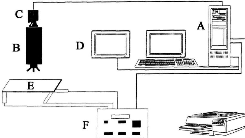
**Figure 2.** The principal components of the Image Analysis System: A PC-486 computer with a frame grabber, B optical microscope, C video camera, D image display monitor, E motorised stage, F stage controller
