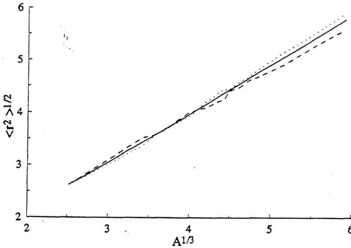
Figure 1 A schematic comparison of  $\langle r^2 \rangle_m^{1/2}$  (solid line),  $\langle r^2 \rangle_n^{1/2}$  (dotted line) and  $\langle r^2 \rangle_p^{1/2}$  (dashed line), as functions of  $A$ , using equations (10) and (11) (see text).
