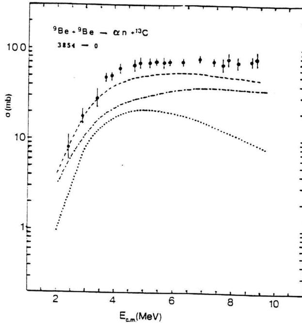
Fig. 2. Excitation function for the  $^{13}\text{C}$ , 3854 KeV  $\gamma$  ray in the  $\alpha$ -transfer channel. The various lines represent theoretical predictions from statistical model calculations (dotted-dashed line), from DWBA calculations (dotted line) and both statistical and DWBA calculations (dashed line) normalized to the data at low energies.
