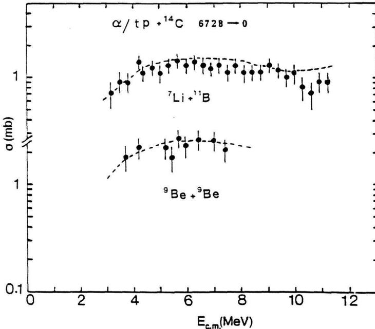
Fig. 1. Excitation function for the 6728 KeV transition of  $^{14}\text{C}$  produced by the  $^7\text{Li}+^{11}\text{B}$  and  $^9\text{Be}+^9\text{Be}$  reactions. The dashed lines are the corresponding theoretical predictions from statistical model calculations using the code STAPRE.
