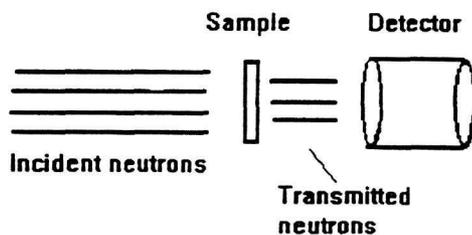
Figure 1: Principle of a transmission experiment
