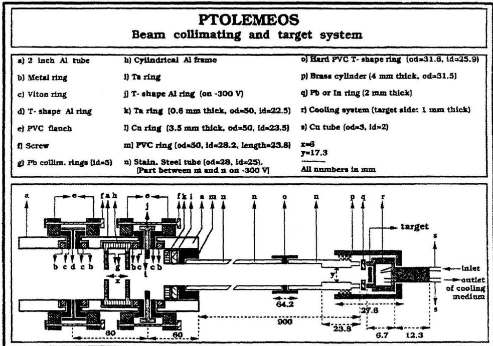
FIG. 9: The target system designed for PTOLEMEOS
