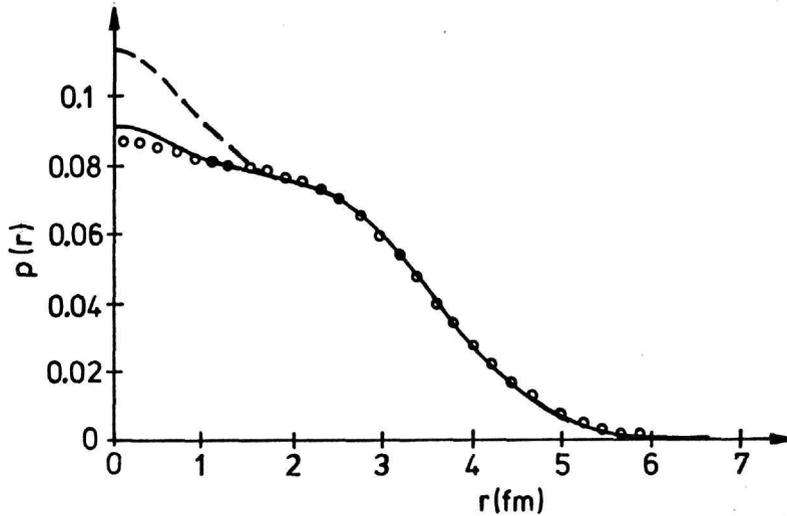
Fig. 1. Plot of the proton density distribution in  $^{40}\text{Ca}$  as calculated with the simple harmonic oscillator shell model (dashed-line) and with eq. (11) by assuming fractional occupation probabilities (solid line). The experimental data (circles) of ref. [10] are also shown.
