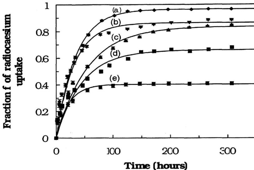
Fig. 1. Kinetics of radiocaesium uptake from aqueous solution  $^{137}\text{Cs}$ :  $1.7 \times 10^{-11}$  M and H:  $2 \times 10^{-4}$  M by (a) 150 mg; (b) 100 mg; (c) 60 mg; (d) 30 mg and (e) 10 mg of ATHINA-A. (Curves represent the fit of the experimental data in eqn (1)).
