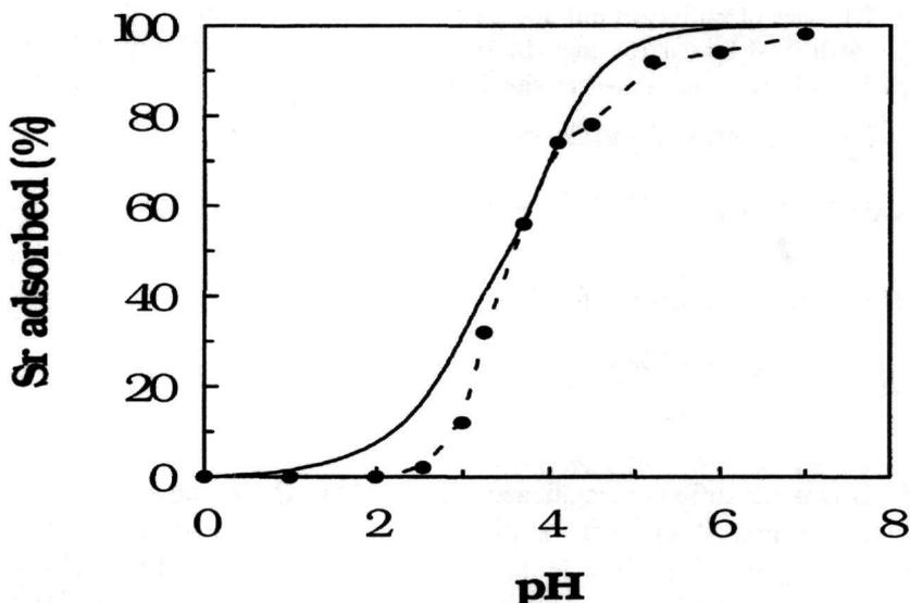
Fig. 2. Influence of pH in strontium sorption on 30 mg of ATHINA-A. The solid line represents the values that the NPL model predicts with  $k(\text{Sr}/\text{H})=9$  ( $\text{pH}=3.7$ ). (Strontium concentration  $1.7 \times 10^{-11}$  M).
