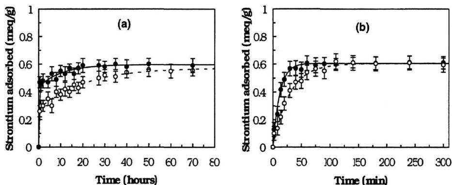
Fig. 3.  $\text{Sr}^{2+}$  exchange kinetics on AZA-D (open circles, dashed line) and FRAZA-D (black circle, solid lines) under (a) static and (b) dynamic experimental conditions. (Strontium concentration was  $0.5 \times 10^{-3}$  M and  $\text{pH} \approx 6.00$ . Grain sizes  $< 45 \mu\text{m}$  were used for both the materials in the dynamic conditions).
