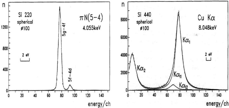
Fig. 2. a) Spectrum of the 5→4 transitions in pionic nitrogen. Ten channels correspond to 1.46 eV b)  $K\alpha_{1,2}$  fluorescence spectrum of Cu. The energy of the diagram line  $K\alpha_{11}$  is 8047.837(2) eV [13]. correspond to 2.81 eV.
