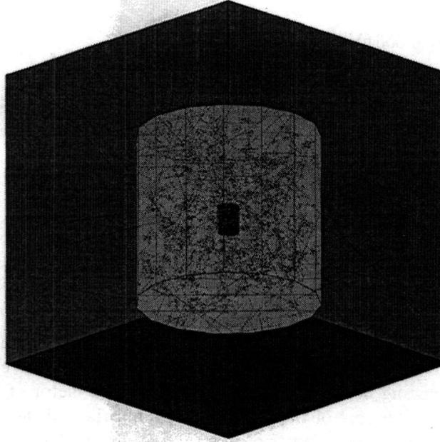
Fig. 7. Simplified model of the GENIUS experiment: 288 enriched  $^{76}\text{Ge}$  detectors with a total of one ton mass in the center of a 12 m high liquid nitrogen tank with 12 m diameter; GEANT Monte Carlo simulation of 1000 2.6 MeV photons randomly distributed in the nitrogen is also shown
