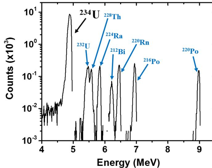
**Figure 3.** A typical spectrum of the  $\alpha$ -activity emitted from the  $^{234}\text{U}$  sample. Apart from the main  $\alpha$ -peak at  $\sim 4.8$  MeV, some other peaks also exist that are attributed to several daughter nuclei (the origin for each one of them is marked), due to the decay chain of  $^{234}\text{U}$ . However, these impurities were found to be much less than 1% of the total active mass.
