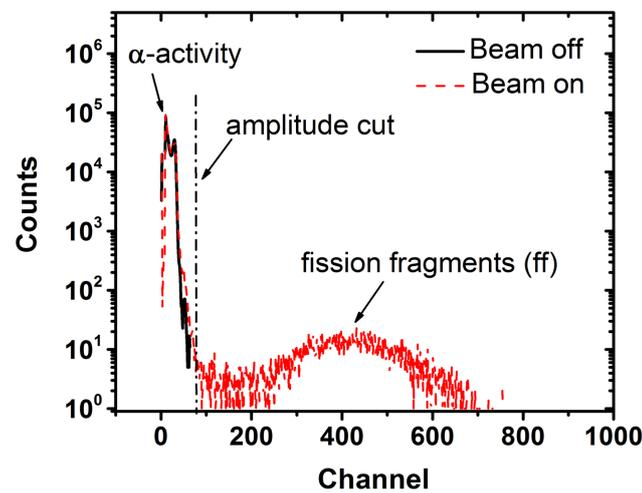
**Figure 7.** Experimental spectrum of the  $^{238}\text{U}$  target obtained using a Micromegas detector. The black solid line corresponds to the  $\alpha$ -activity of the target (Beam off), while the red dashed one (Beam on) is the spectrum that was obtained during the irradiation at  $(16.5 \pm 0.3)$  MeV. On the latter, apart from the peak of the  $\alpha$ -background activity, also the peak of the fission fragments is present.
