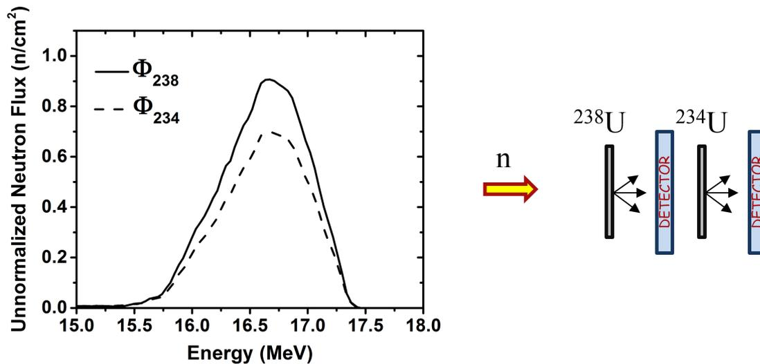
**Figure 5.** (Left) The results of the MCNP5 simulation for the neutron flux with respect to the neutron energy in both the reference ( $^{238}\text{U}$ ) and measured ( $^{234}\text{U}$ ) targets, for the irradiation at  $(16.5 \pm 0.3)$  MeV. As shown in the schematic representation (Right), the  $^{238}\text{U}$  target was placed in front of the  $^{234}\text{U}$  one, with respect to the neutron beam.
