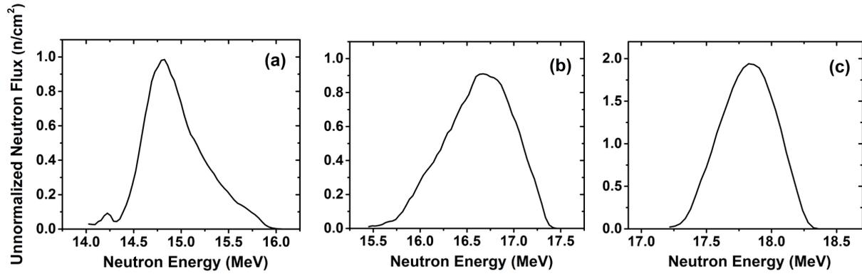
**Figure 4.** Unnormalized neutron flux for the three irradiations at (a)  $(14.8 \pm 0.3)$ , (b)  $(16.5 \pm 0.3)$ , and (c)  $(17.8 \pm 0.2)$  MeV, as obtained by coupling the NeuSDesc and MCNP5 codes. The figures are focused on the main neutron energy region, to highlight the FWHM of each neutron peak from which the neutron energy uncertainty was estimated.
