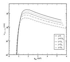
Figure 2. Momentum dependence of the effective DBHF cross section at various baryon densities  $\rho$  (in units of the saturation density  $\rho_0 = 0.1854 \ fm^{-3}$ ).
