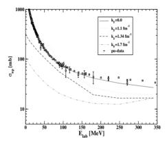
Figure 1. Elastic in-medium neutron-proton cross sections at various Fermi momenta  $k_F$  as a function of the laboratory energy  $E_{lab}$ . The free cross section ( $k_F = 0$ ) is compared to the experimental total np cross section [12].
