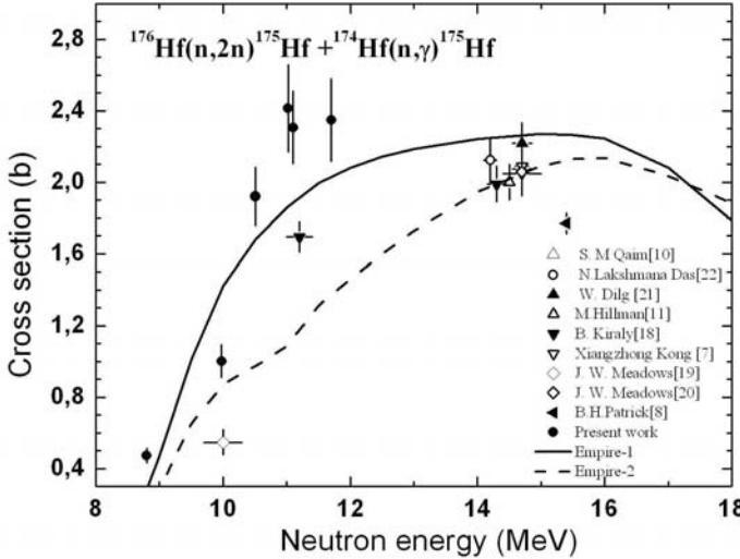
Figure 3. Comparison between measured cross sections and theoretical predictions for the  $^{176}\text{Hf}(n,2n)^{175}\text{Hf}$  reaction. The circles represent the values of the present work and include contribution from the  $^{174}\text{Hf}(n,\gamma)^{175}\text{Hf}$  reaction, while the other experimental data have been taken from literature. The solid and dashed lines correspond to calculations performed using the code EMPIRE-II with different NLDs (see the text).
