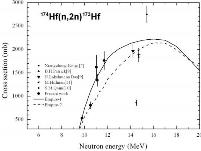
Figure 2. Comparison between measured cross sections and theoretical predictions for the  $^{174}\text{Hf}(n,2n)^{173}\text{Hf}$  reaction. The circles represent the values of the present work while the other experimental data have been taken from literature. The solid and dashed lines correspond to calculations performed using the code EMPIRE-II with different NLDs (see the text).
