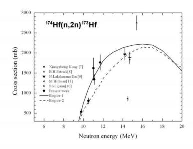
Figure 2. Comparison between measured cross sections and theoretical predictions for the  $^{174}$ Hf(n,2n) $^{173}$ Hf reaction. The circles represent the values of the present work while the other experimental data have been taken from literature. The solid and dashed lines correspond to calculations performed using the code EMPIRE-II with different NLDs (see the text).
