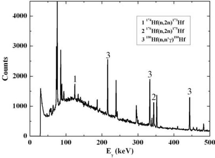
Figure 1. Typical off line spectrum of natural  $\text{HfO}_2$  taken at neutron energy 11.1 MeV.
