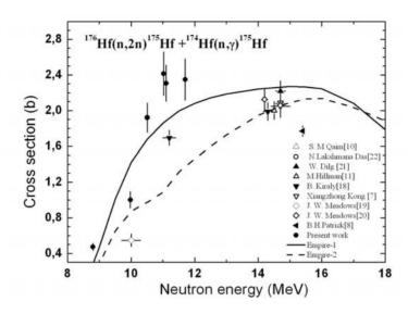
Figure 3. Comparison between measured cross sections and theoretical predictions for the  $^{176}$ Hf(n,2n) $^{175}$ Hf reaction. The circles represent the values of the present work and include contribution from the  $^{174}$ Hf(n, $\gamma$ ) $^{175}$ Hf reaction, while the other experimental data have been taken from literature. The solid and dashed lines correspond to calculations performed using the code EMPIRE-II with different NLDs (see the text).
