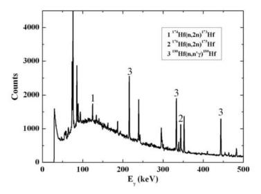
Figure 1. Typical off line spectrum of natural HfO<sub>2</sub> taken at neutron energy 11.1 MeV.
