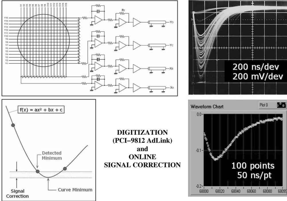
Figure 1. *Upper part:* Wiring scheme for the 16+16 anode signals of the HAMAMATSU R2486 Photomultiplier tube through the resistive chain and the four charge preamplifiers. The analog signal output for a typical CsI(Tl) scintillator is shown in the right figure. *Lower part:* Signal sampling after digitization with the PCI-9812 card and the principle of the 2<sup>nd</sup> order correction algorithm for the location of the minimum.
