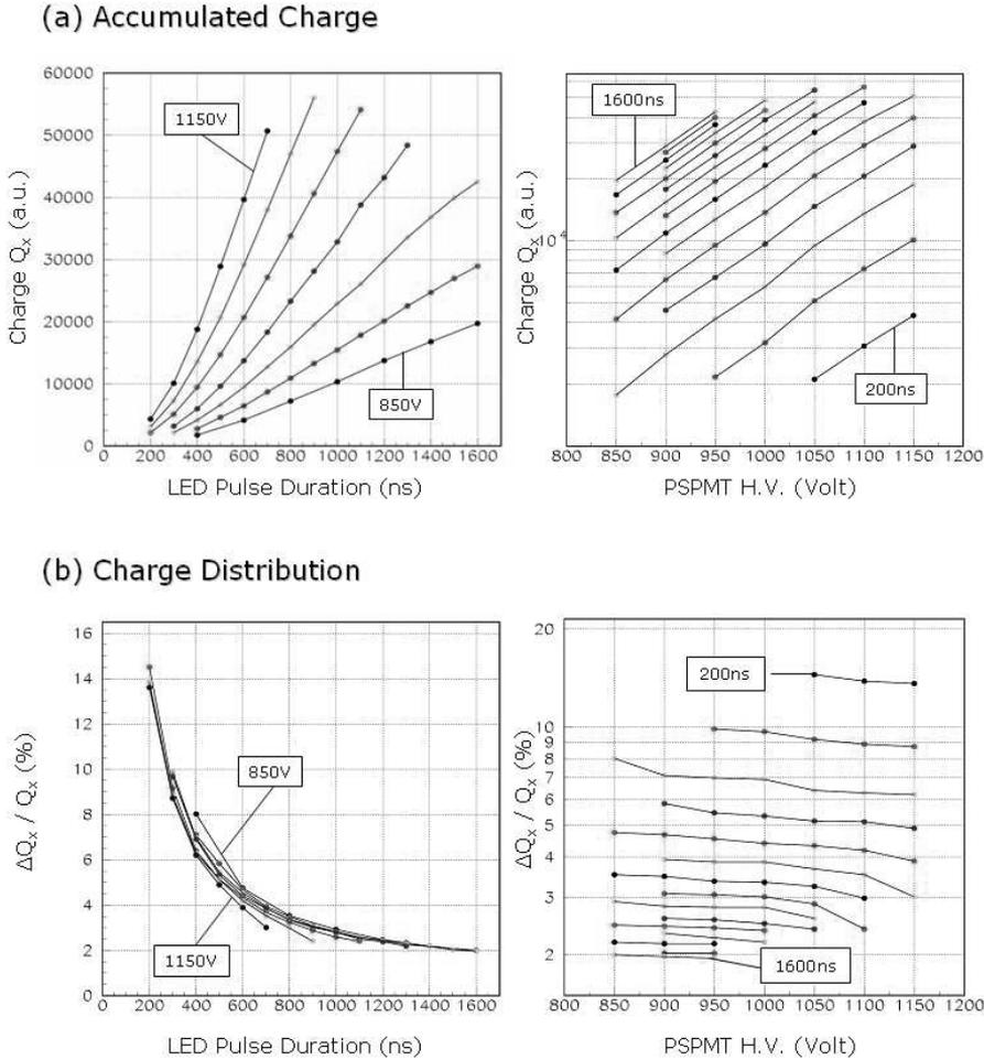
Figure 3. Accumulated charge  $Q$  and relative charge distribution  $\Delta Q/Q$  of the x-group wires of the PSPMT for the High Voltage operation range 850 V – 1150 V (in steps of 50 V) and LED pulse duration range 200 ns – 1600 ns (in steps of 100 ns). Similar curves are also obtained for the y-group wires.
