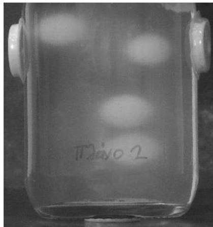
Figure 2. A photograph of the gel vial irradiated with the Leksell gamma knife unit using a GammaPlan generated plan resembling treatment of four metastases with four different shots.
