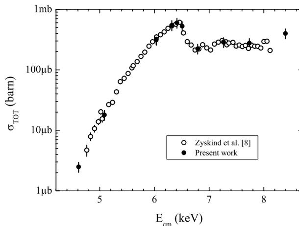
Figure 5. Cross section measurements of the  $^{62}\text{Ni}(\alpha, \gamma)^{66}\text{Zn}$  reaction. The black dots represent the results of the present work while the open circles correspond to the results of the previous work of Zyskind *et al.* [8].
