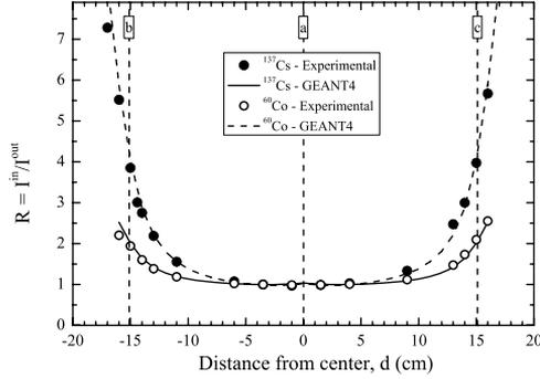
Figure 3. In/out ratio  $R$  obtained with a  $^{137}\text{Cs}$  source (open circles) and a  $^{60}\text{Co}$  source (black dots) at various distances from the center of the detector along the bore hole axis. The solid curves are the result of the corresponding GEANT4 simulations.
