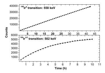
Figure 2. The evolution of the photopeak net area counts with measuring time. The experimental data (points), as resulted after the 10.5 irradiation, are presented with the theoretical fitted curve for the expected half-life time (line). The above panel corresponds to the 558 keV transition from the decay of the ground state (g) and the lower panel to the 502 keV transition form the decay of the second isomeric state (m2).
