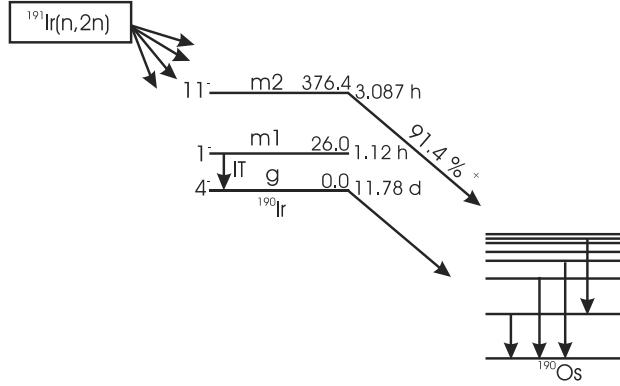
Figure 1. Simplified representation of formation and decay of the ground state and isomeric states of  $^{190}\text{Ir}$ . All energies are in keV
