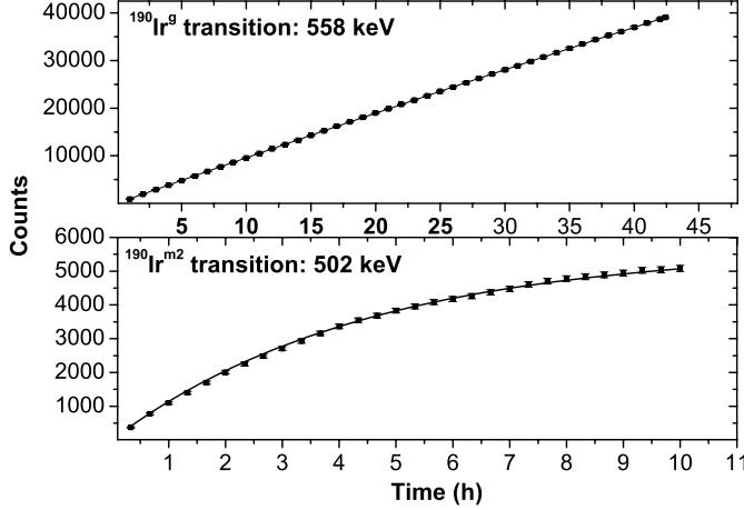
Figure 2. The evolution of the photopeak net area counts with measuring time. The experimental data (points), as resulted after the 10.5 irradiation, are presented with the theoretical fitted curve for the expected half-life time (line). The above panel corresponds to the 558 keV transition from the decay of the ground state (g) and the lower panel to the 502 keV transition from the decay of the second isomeric state (m2).
