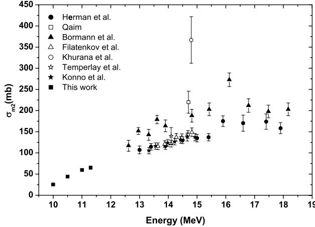
Figure 4. The measured cross section  $\sigma_{m2}$  for the population of the second isomeric state of  $^{190}Ir$
