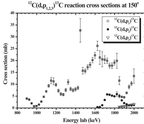
Figure 2. Differential cross section spectra (mb/sr) of the  $^{12}\text{C}(\text{d},\text{p}_{1,2,3})^{13}\text{C}$  reactions at  $150^\circ$  for  $E_{d,lab}=900$ -2000 keV.
