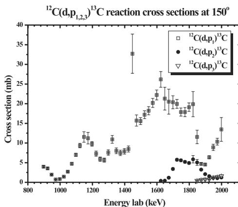
Figure 2. Differential cross section spectra (mb/sr) of the  $^{12}\text{C}(d,p_{1,2,3})^{13}\text{C}$  reactions at  $150^\circ$  for  $E_{d,lab}=900-2000$  keV.
