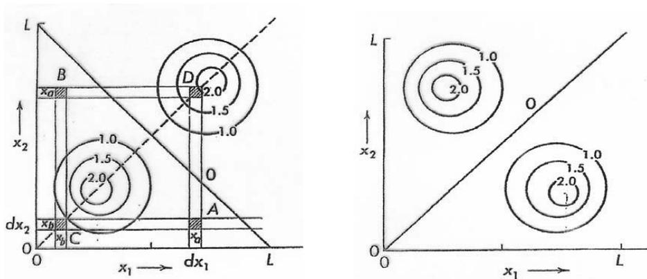
**Fig.1.** (a) Symmetric wave function:  $\psi_s^* \psi_s$  with  $n = 1$  and  $k = 2$ , according to Eq.(10), (b) Antisymmetric wave function:  $\psi_a^* \psi_a$  with  $n = 1$  and  $k = 2$ , according to Eq.(11).
