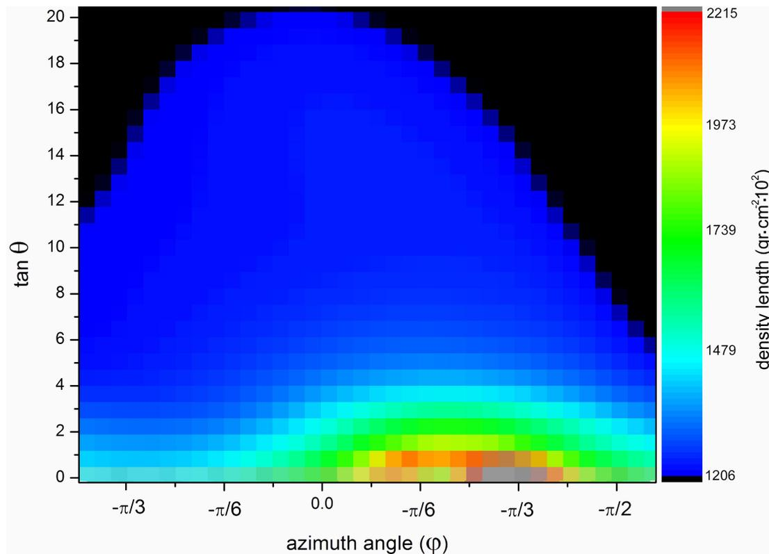
**Figure 10.** Density length model of the volcanic dome of Methana concerned here. Color-graded scale on the right provides the density length estimates ( $\text{gr}\cdot\text{cm}^{-2}\cdot 10^{-3}$ ) in the  $(\varphi, \theta)$  direction.
