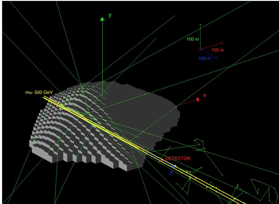
**Figure 4.** Schematic illustration of the simulation framework of the volcanic dome of Methana in Geant4. Yellow lines correspond to muon trajectories while jagged green lines represent photon tracks due to Compton scattering. X axis points East.
