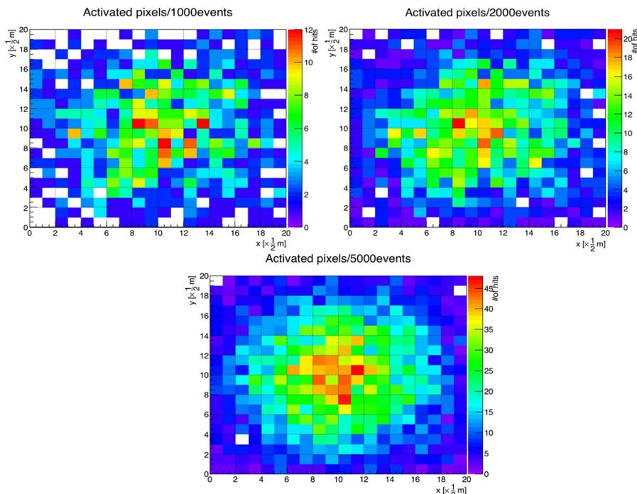
**Figure 9.** Count distribution on the MicroMegas detector of 1000 (top left), 2000 (top right) and 5000 (bottom) muons injected at 900 GeV. Resolution set to  $0.5 \times 0.5$  m. (y,x axes in meters; number of muon hits represented as colors)
