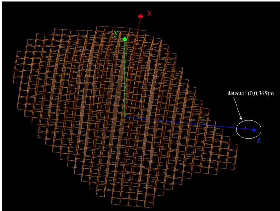
**Figure 3.** Model of the volcanic dome of the Methana volcano consisted of parallelepiped physical volumes (voxels) in the Geant4 computational region. X-axis (up) points East. The detector is placed south of the dome.
