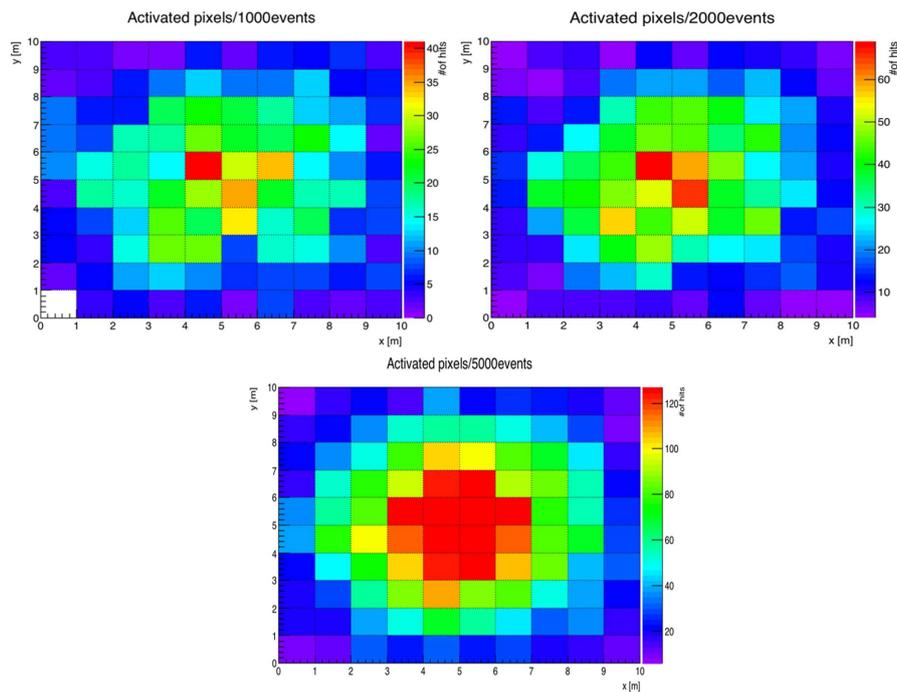
**Figure 8.** Count distribution on the MicroMegas detector of 1000 (top left), 2000 (top right) and 5000 (bottom) muons injected at 900 GeV. Resolution set to  $1 \times 1$  m. (y,x axes in meters; number of muon hits represented as colors)
