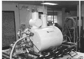
Figure 4. Portable antiproton trap, able to transfer  $10^{12}$  antiprotons.
