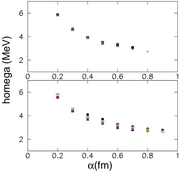
Fig. 1. The evolution of the barrier curvature ( $\hbar\omega$  as a function of the potential diffusivity for  ${}^6\text{Li}+{}^{28}\text{Si}$  (top) and  ${}^7\text{Li}+{}^{28}\text{Si}$  (bottom), at several barrier energies.
