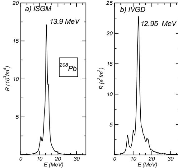
Fig. 3. The isoscalar monopole (a), and the isovector dipole (b) strength distributions in  $^{208}\text{Pb}$  calculated with the effective interaction NL3\*. The experimental excitation energies are:  $14.1 \pm 0.3$  MeV for the monopole resonance, and  $13.3 \pm 0.1$  MeV for the dipole resonance, respectively.
