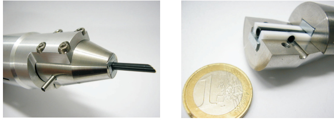
Fig. 3. Nozzle for the low-energy Si(Li) detector including deflections magnets and channel for constant Helium flow.
