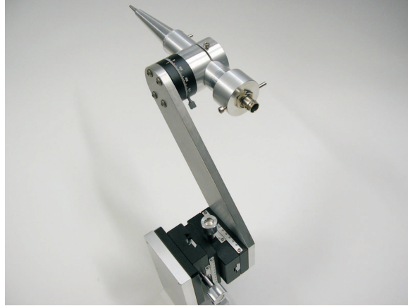
Fig. 4. Conical vacuum chamber for the surface barrier detector utilized in RBS measurements.
