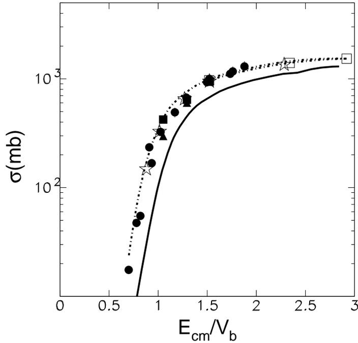
Fig. 1. Total reaction cross sections for  ${}^6\text{Li}+{}^{28}\text{Si}$  are compared well with CDCC calculations, designated with the dotted-dashed line. These results are also compared with BPM calculations according to Wong [1] and show a large enhancement.
