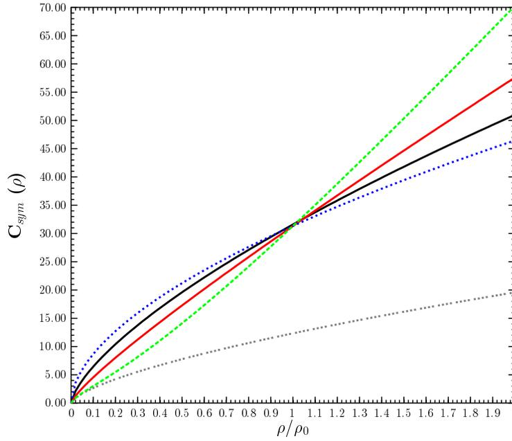
Fig. 1. (Color Online) Density dependence of the nuclear symmetry energy  $C_{sym}(\rho)$  corresponding to the forms of the nucleon-nucleon symmetry potential in the CoMD code. Blue (dotted): asy-soft, red (solid): asy-stiff, green (dashed): super asy-stiff and grey (lower dotted) line: no symmetry potential. The black (solid) line represents the form  $31.6(\rho/\rho_0)^{0.69}$  consistent with the isoscaling analysis of fragments from central heavy-ion collisions [2].
