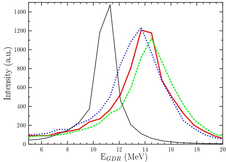
Fig. 7. (Color Online) Giant dipole resonance (GDR) response of an isolated  $^{86}\text{Kr}$  nucleus predicted by CoMD. The various lines correspond to the choices of the nucleon symmetry potential as follows: blue (dotted): asy-soft, red (solid): asy-stiff, green (dashed): super asy-stiff, and black (left solid): no symmetry potential. The expected value of the energy according to the empirical GRD systematics is 16.8 MeV [15,16].
