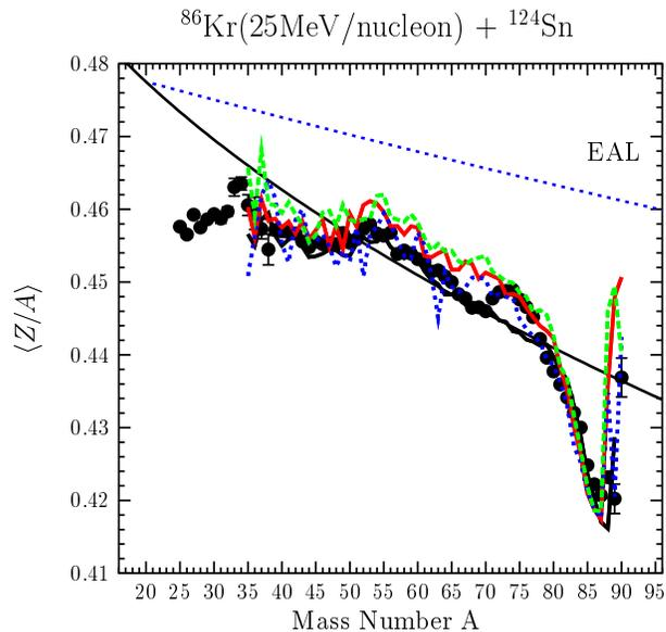
Fig. 4. (Color Online) Mean projectile residue  $Z/A$  as a function of residue mass for the reaction  $^{86}\text{Kr}(25\text{MeV/nucleon}) + ^{124}\text{Sn}$ . DIT calculations are given by the black (solid) line that traces the data. CoMD calculations are given by the other three lines as in Fig. 2 (see text). Black points: MARS data [3]. Black near-diagonal (solid) line: stability line. EAL: evaporation attractor line [14].
