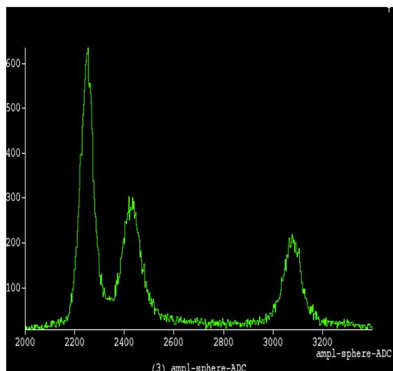
**Figure 5.** The peaks observed from a  $^{222}\text{Rn}$  radioactive source. From left to right we observe the  $^{222}\text{Rn}$  peak at 5.5 MeV, the  $^{218}\text{Po}$  and  $^{214}\text{Po}$  at 6.0 MeV and 7.7 MeV respectively.
