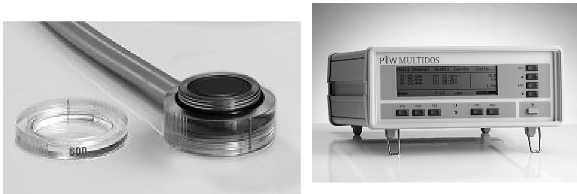
Figure 2: Markus ionization chamber – MULTIDOS electrometer
