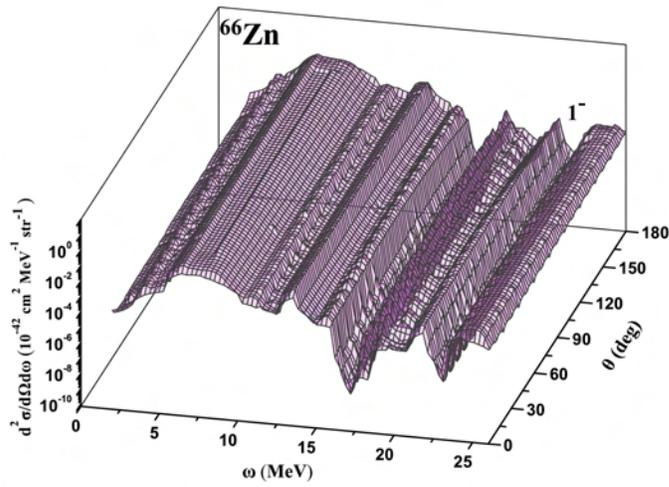
Fig. 2. The double differential cross section,  $d^2\sigma/d\Omega d\omega$  as function of the excitation energy  $\omega$  of the nucleus and the scattering angle  $\theta$  of the outgoing lepton, for  $^{66}\text{Zn}$ . The incoming neutrino energy is  $\varepsilon_\nu = 40$  MeV. The curves correspond to the principal multipolarity  $J^\pi = 1^-$ .
