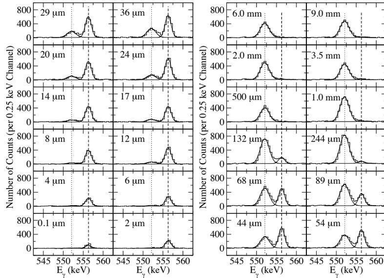
Figure 2: Deconvoluted spectra for all separate target-stopper distances of the stopped and backward-shifted component of the 556-keV,  $I^\pi = 2_1^+ \rightarrow 0_1^+$  transition, from a gate placed on the forward-shifted component of the 719-keV,  $I^\pi = 4_1^+ \rightarrow 2_1^+$  transition. The centroids of the stopped and backward-shifted peaks are shown by the dashed and dotted lines respectively.
