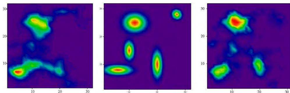
Figure 4: Reconstruction of a  $32 \times 32$  software phantom (shown in the middle) with the ANN technique and for  $M = 18$  projections. *Left*: One hidden layer with 64 nodes is used *Right*: No hidden layer used.
