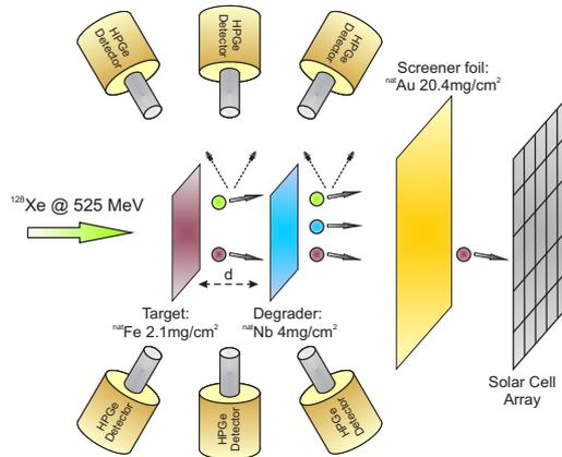
Figure 1: The experimental setup for the Coulex-Plunger technique is shown in the figure. The array of solar cells was placed at the endcap of the beamline covering an angular span between  $8^\circ$  and  $35^\circ$  around the beam axis. This allowed the detection of the Fe recoils which gave a clear trigger for the reaction.
