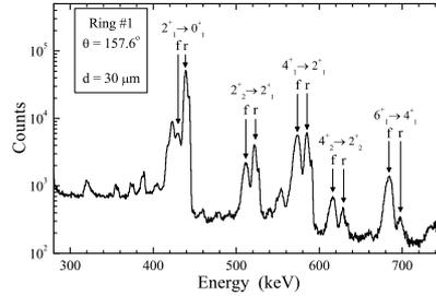
Figure 2: A typical RDDS spectrum is shown. Marked with “f” and “r” are the “flight” and “retarded” component accordingly of each of the five strongest transitions of the Coulomb excited  $^{128}\text{Xe}$ . The spectrum is taken at an intermediate plunger distance of  $30\mu\text{m}$  therefore both shifted and unshifted components are clearly visible.
