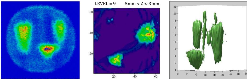
Fig. 3. *Left:* Planar image taken with the  $\gamma$ -Camera at  $15^\circ$  angle. *Center:* Reconstructed  $64 \times 64$  matrix of the  $9^{th}$  slice (out of 21) at  $Z = -4.00 \pm 2.0 \text{ mm}$  using all planar images. *Right:* The obtained 3D tomographic image of the gel-phantom by contour plotting all the 21 reconstructed tomograms.
