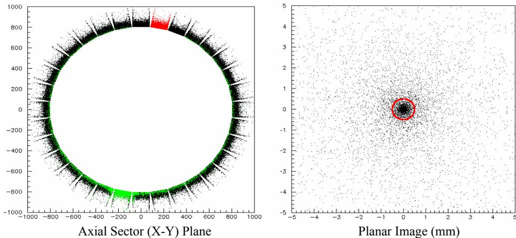
Fig. 3. *Left:* The axial (X-Y) reconstructed image of coincidence events detected by the simulated PET ring system. Coincident events detected within the first sector are shown in different color. *Right:* Planar image of a  $^{18}\text{F}$ -positron emitter point source.
