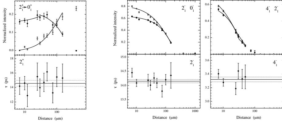
Fig. 3. The  $\tau$ -plots that resulted from the coincidence (left) and the singles (right) analysis are shown in the figure. For the fitting of the decay curves and the extraction of the lifetimes, the computer program NAPATAU [16] was used.
