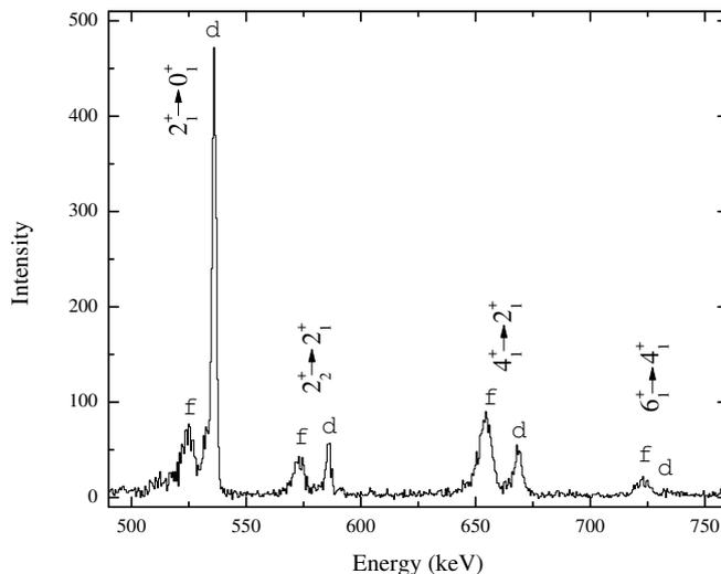
Fig. 2. A typical particle gated  $\gamma$ - $\gamma$ -spectrum is shown where the four strongest transitions of the Coulomb excited  $^{130}\text{Xe}$  are indicated. Marked with “f” and “d” are the “flight” and “degraded” components of each transition. The spectrum is taken at an intermediate plunger distance of  $30\ \mu\text{m}$  therefore both shifted and unshifted components are clearly visible.
