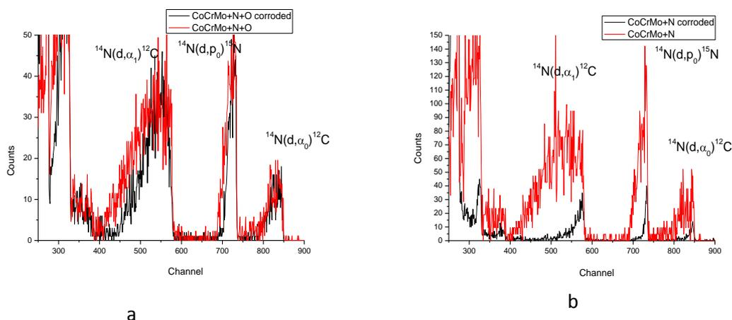
Fig. 1: NRA spectra of the CoCrMo+N+O and CoCrMo+N samples prior and after the corrosion testing in 0.9% NaCl solution.
