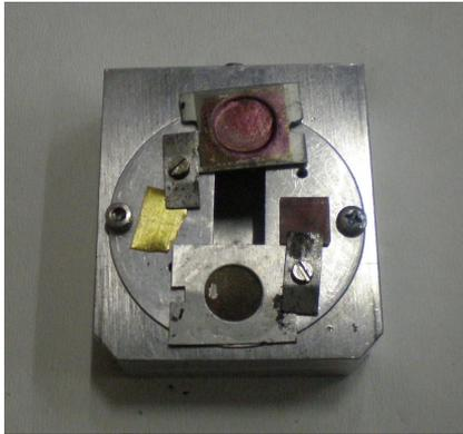
Figure 1: A sample holder with mounted LiF and <sup>nat</sup>C targets. A gold foil (left) was used as current calibration.
