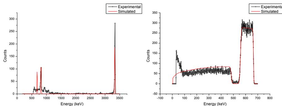
Figure 3: *Left:* A typical spectrum of a thin  $^{nat}\text{C}$  bombarded with deuterons of  $E_d = 1550$  keV acquired at an angle of  $150^\circ$  *Right:* A typical spectrum of a  $^{nat}\text{Ti}$  thin film irradiated with a proton beam of  $E_p = 1500$  keV at  $150^\circ$
