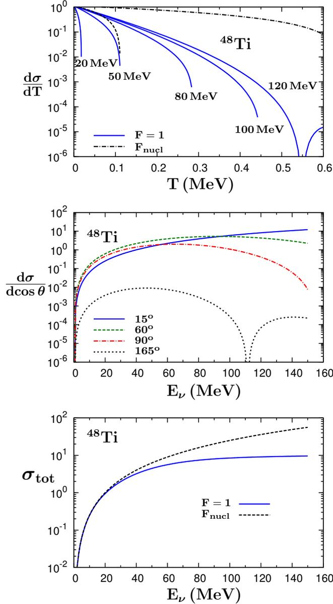
Fig. 2. *Top:* The differential cross section  $d\sigma/dT$  (in units  $10^{-37} \text{cm}^2/\text{MeV}$ ) as a function of the nuclear recoil energy  $T$  for various neutrino energies.  $d\sigma/dT$  is compared to that of point-like nucleus ( $F = 1$ ) for  $E_\nu = 50 \text{ MeV}$  and  $E_\nu = 120 \text{ MeV}$ . For rather low energies the results coincide, however for intermediate or high energies this is not the case.
