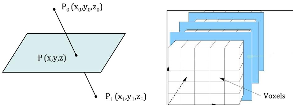
Fig. 1. *Left:* Intersection of the annihilation line defined by the two opposite 511-keV photons detected at  $P_0(x_0, y_0, z_0)$  and  $P_1(x_1, y_1, z_1)$  respectively with a plane. *Right:* Definition of the voxelized volume of interest.
