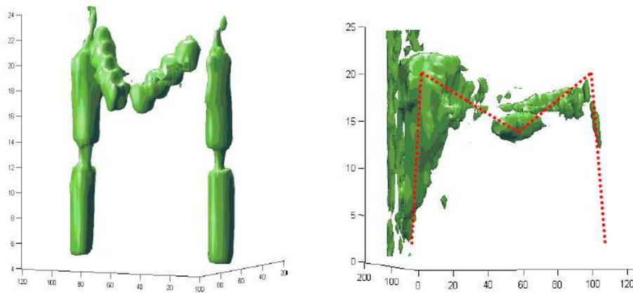
Fig. 4. *Left*: 3D reconstruction (ISO-Value=0.19) for a temperature of  $36.5^{\circ}\text{C}$  corresponding to a resistor current of  $I = 40\text{ mA}$  (non absorbing medium). *Right*: 3D reconstruction (ISO-Value=0.07) for a temperature of  $49.5^{\circ}\text{C}$  corresponding to a resistor current of  $I = 80\text{ mA}$  (agarose absorbing medium). The images were created by contour plotting all the obtained tomograms of the reconstruction process using the MATLAB package.
