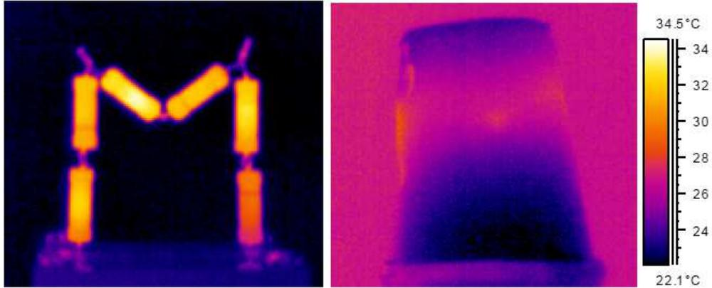
Fig. 3. *Left*: Planar images (no absorbing medium) obtained with the thermal camera. *Right*: Planar images obtained in the agarose absorbing medium with the thermal camera. The different colors depicted in the images indicate different temperatures emitted by the phantom. The fact that the emitted infrared radiation is a function of the phantom's surface temperature makes it possible for the camera to calculate those temperatures.
