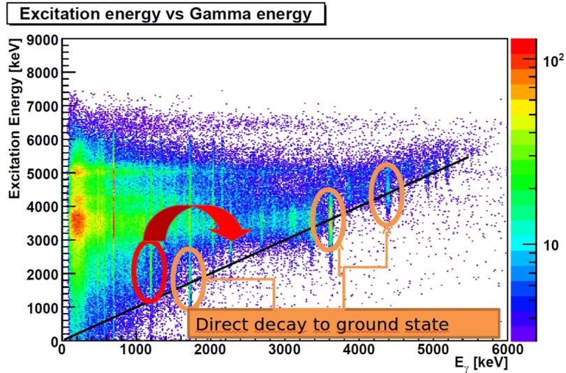
Fig. 2. The excitation energy of the residual nucleus ( $^{67}\text{Ni}$ ) as deduced from the kinetic energy of the protons plotted together with the  $\gamma$ -ray energy detected in coincidence with the protons. The transitions that de-excite directly to the ground state are lying across the diagonal (black line). Other populated levels that deexcite through an intermediate level are lying above the diagonal (e.g. the 2.2 MeV state indicated with the red circle).
