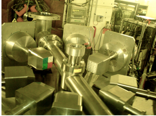
Figure 1: The experimental setup comprising eight EXOGAM segmented detectors
