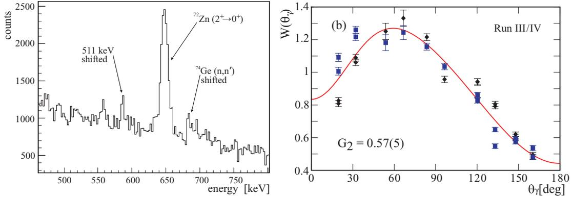
Figure 2: *Left*: Doppler-corrected random-subtracted  $\gamma$ -ray spectrum near the  $^{72}\text{Zn} (2^+ \rightarrow 0^+)$  line. *Right*: Laboratory frame angular correlations for the combined fit for  $^{76}\text{Ge}$  in Gd (black diamonds), and  $^{72}\text{Zn}$  in Gd (blue squares).
