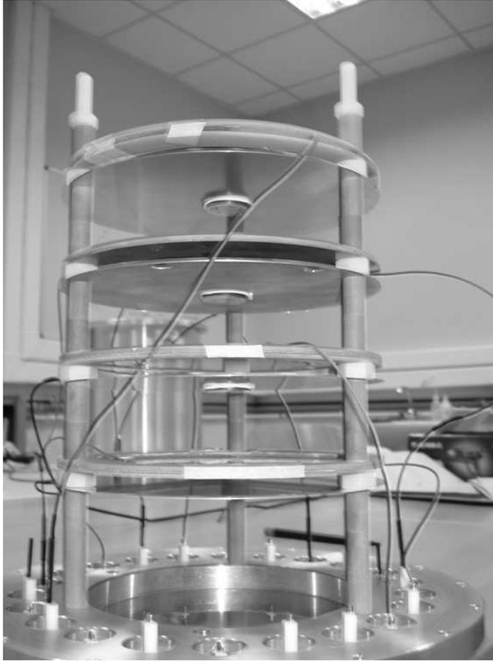
Fig. 1. Photo of the MicroMegas detector assembly.
