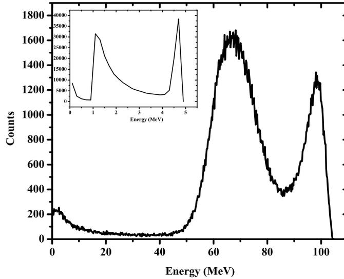
Fig. 2. The simulated energy deposition of the fission fragments in the gas of the detector, produced by an external source routine and emitted isotropically in the  $^{237}\text{Np}$  target. The inset contains the simulated energy deposition of 4.8 MeV alphas, emitted isotropically in the  $^{237}\text{Np}$  target.
