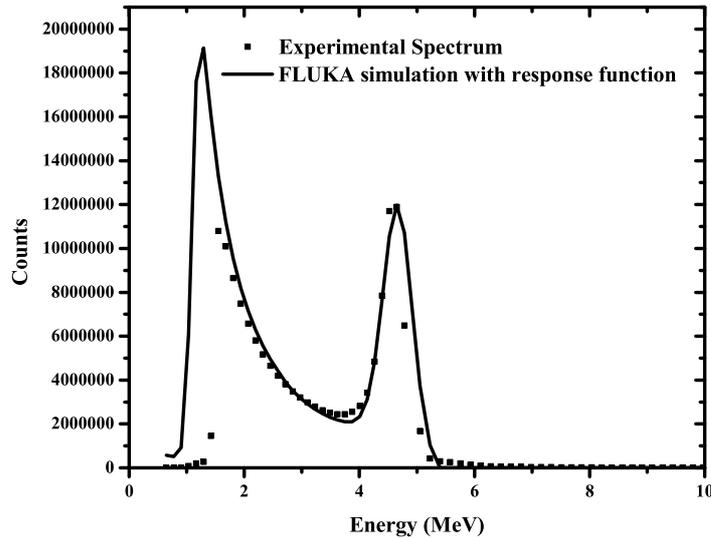
Fig. 3. The comparison of the convoluted with a gaussian resolution function FLUKA histogram with the experimental one for the alphas. The high alpha activity of  $^{237}\text{Np}$  caused pile up of the alpha pulses in the detector, which is not taken into account at the FLUKA simulation. A threshold was applied at the low-energy part of the experimental spectrum.
